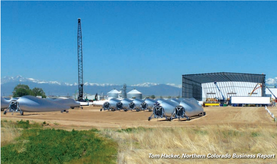
BIG BLADES – Wind turbine blades, each 130 feet long, await shipment by rail from the Vestas Wind Systems plant in Windsor, where an expansion that will double the space is under way.
