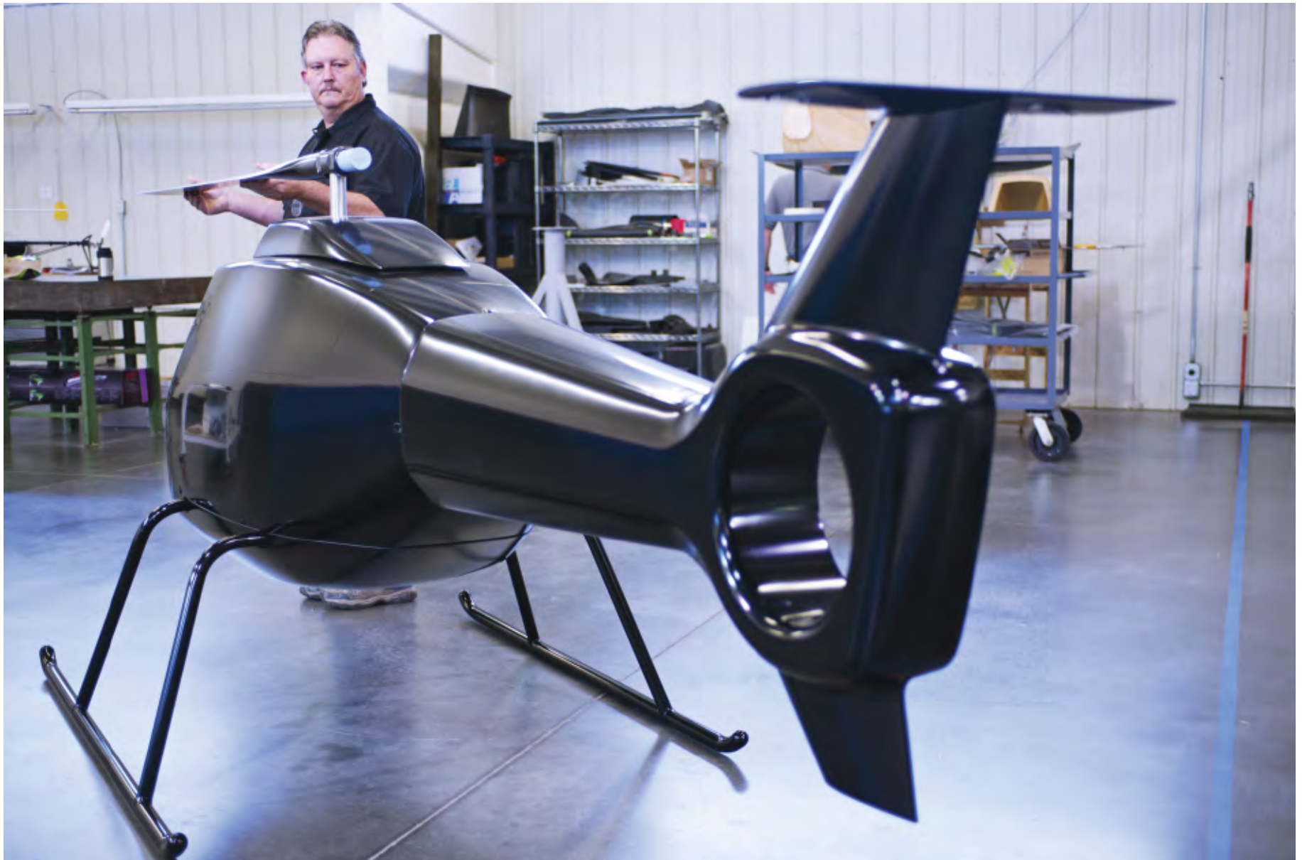
GEARING UP – Composite tech Andrew Simmering attaches the rotor blades on a Scion Aviation Badger.
