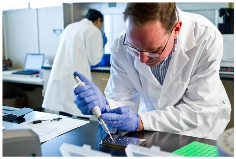
Westen Hahn spots a mass spectrometry plate used to generate a VeriStrat result.
