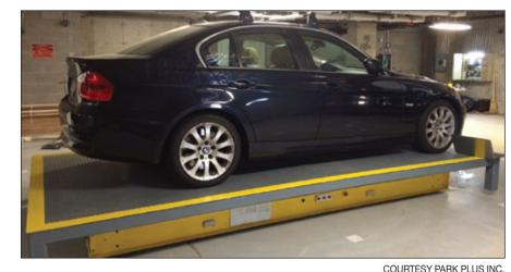
Cars will be placed on a pallet that is powered by a battery-powered, automated guided vehicle. The AGV slides under the pallet, lifts it slightly and travels a preprogrammed route to a parking space.
