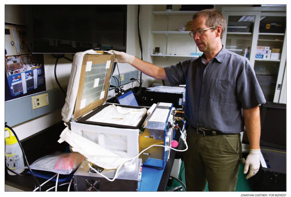
Paul Koenig, Sr. a mechanical design engineer at the University of Colorado's BioServe Space Technologies center, shows off a container used to house experiments being transported into space.
